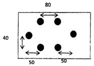
Calculate the maximum tension which the plate can carry in each case. Which arrangement is stronger?
